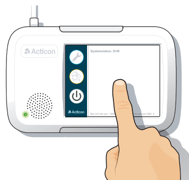
The control panel is activated by pressing the screen. The light-emitting diode (LED) at the bottom left glows green during operation.
