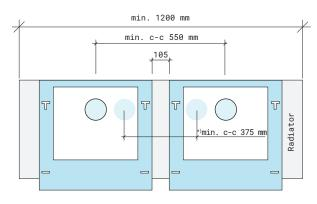
\*) This applies to duct hole with a diameter of Ø100-145 mm and if the holes are eccentrically positioned as shown in the above figure.
