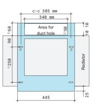
For radiators with a height of 300 mm, the following applies:
